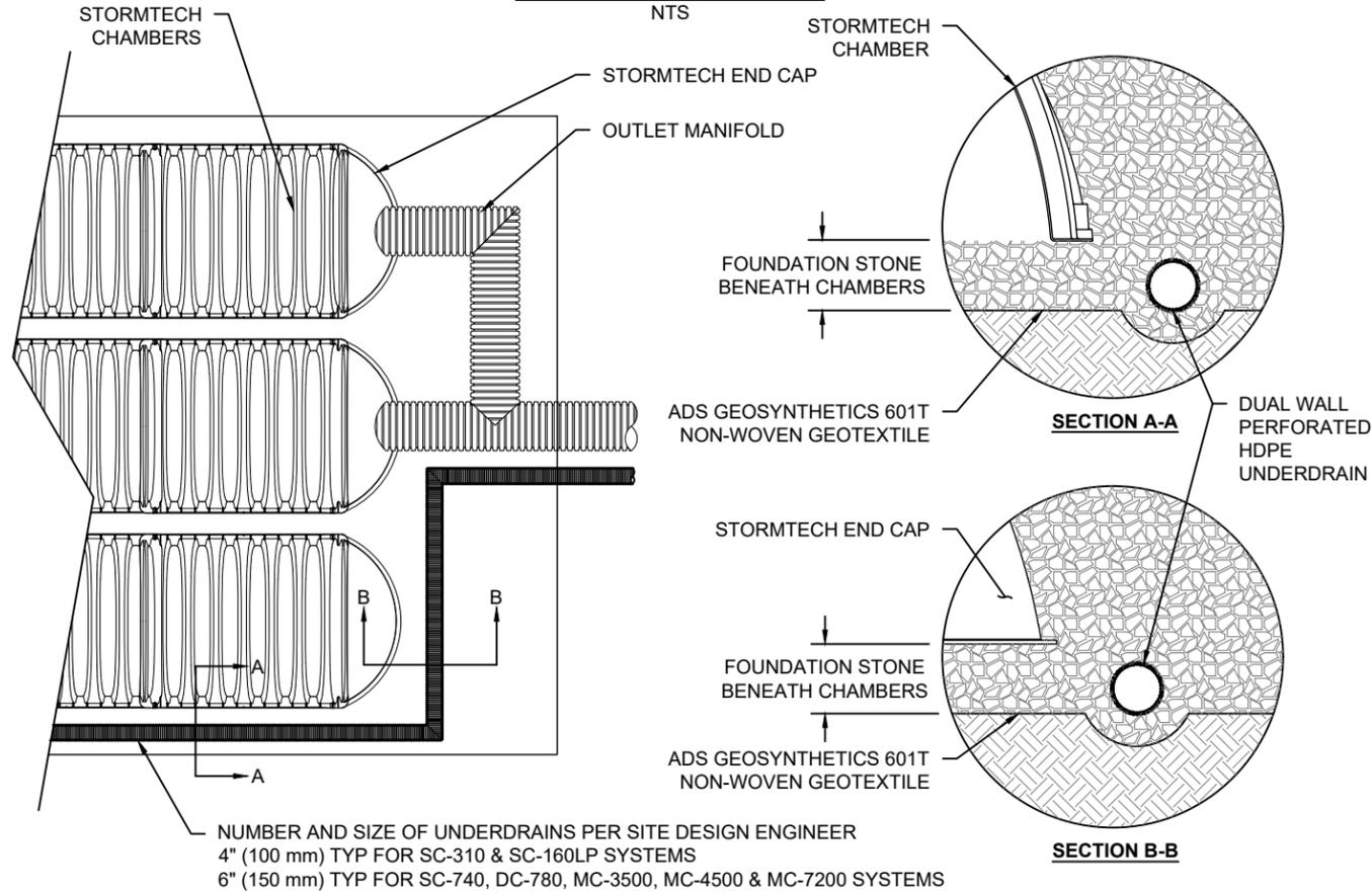
NUMBER AND SIZE OF UNDERDRAINS PER SITE DESIGN ENGINEER
